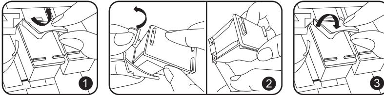
1. Remove the cartridge from the printer when it used up.
